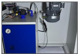
Compact **Built-In Boiler** with a capacity of 4 Kg/ Hr. Placed below the table top inside the cabinet, covered from the front with easy access from the rear. **S.S.304** shell of eight litres with efficient 2Kw heater for maximum output. Comes with safety cap & pressure gauge.
